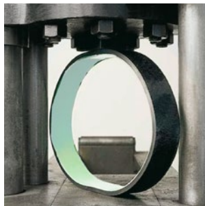
If the pipe becomes deformed, the coating remains intact due to the elasticity of the polyurethane.
