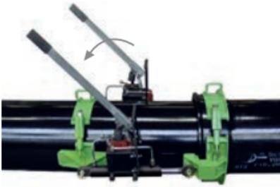
Dismantling push-in joint assembled for a long time: place the thin steel leaves Fig. 255-2 in the gap between the spigot and the socket using hammering accessories Fig. 255-1.
